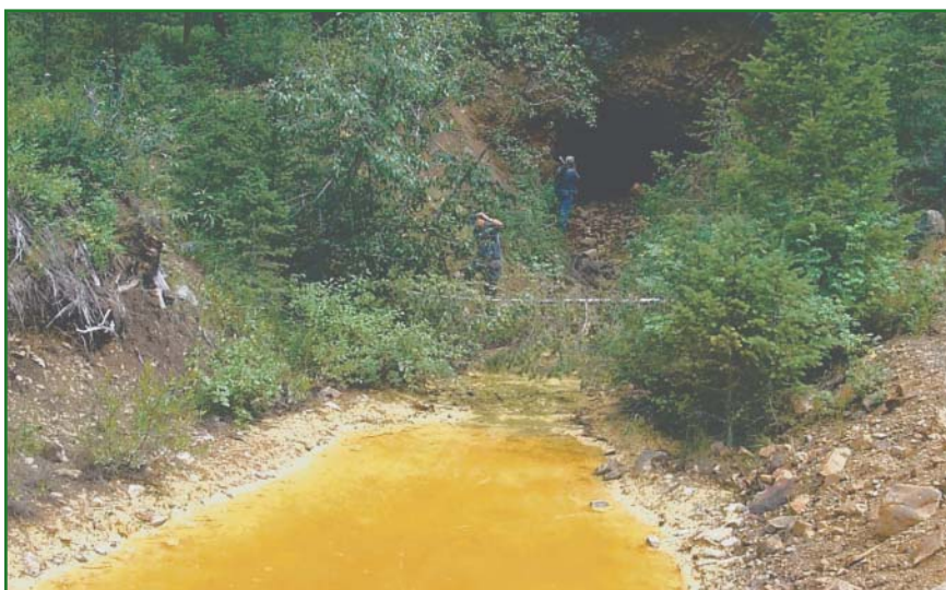
The acid mine discharge at one of the adits at the Charter Oak Mine southeast of Elliston, MT, in the Helena National Forest.
